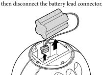
When disconnect the connector, be sure to hold the
